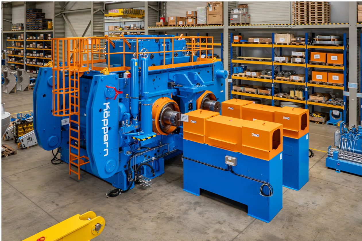
Figure 4: Factory Acceptance Testing of the HPRG tertiary crusher has been completed at the Köppern factory in Germany.
